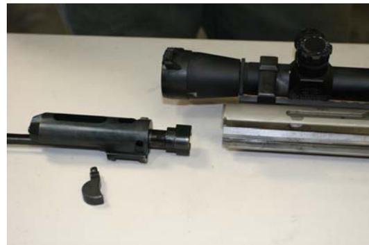
7. To disassemble the Bolt pull the little pin out of the back left side of the Bolt. Be careful not to lose the Firing pin spring when pulling the Firing Pin.
