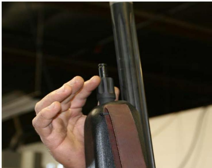
3. Loosen the Montana Sling and slide the front Stock forward towards the muzzle, the sling will pull out of the stock after it clears the retaining rod.
