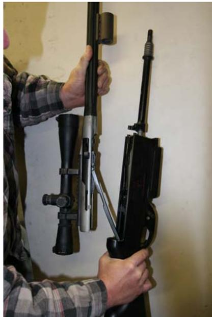
6. To remove the bolt assembly, slide the Bolt handle to where the slot is bigger in the upper receiver. It will pull out of the Main Bolt in this location. It is a little bit of a pull but does not require any tools. Now simply slide the Bolt out the rear of the Upper Receiver.
