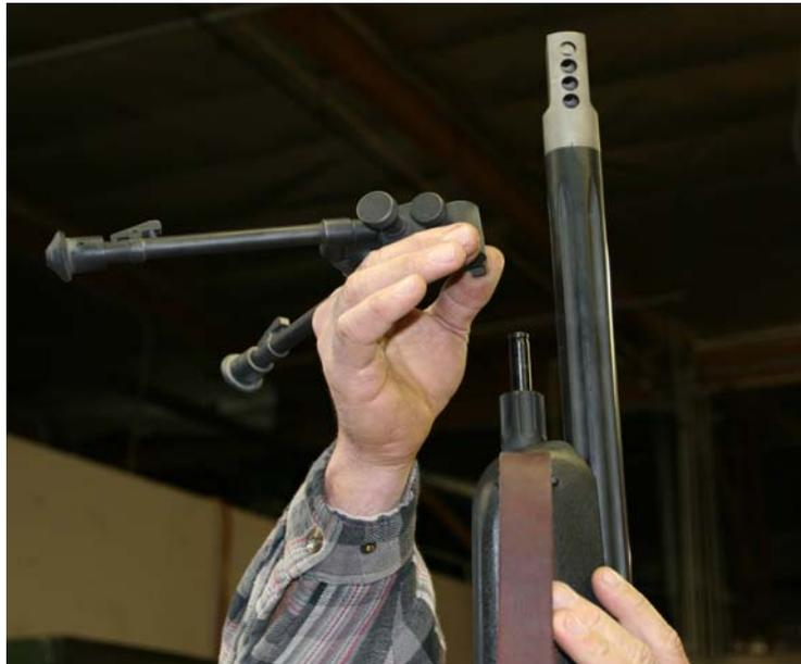
2. Unscrew the front Stock retaining nut; it should only be hand tight.
