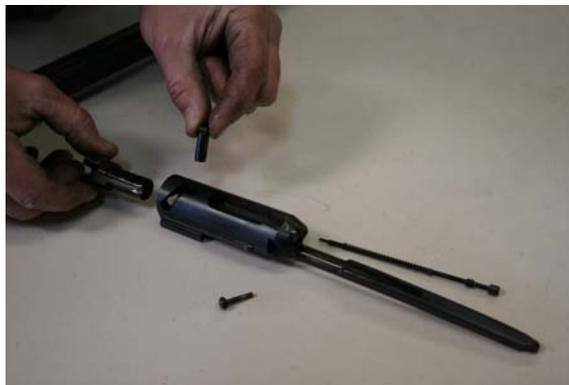
8. Reassembly is easy. The only difference is after you have the upper receiver lined up on the lower receiver and it all looks ready to go back together. Now you have to pull the Bolt handle back about 5/8 of an inch to allow the Bolt to go over the 2 push pins in the lower receiver. After that just follow your steps backwards or your instincts...
